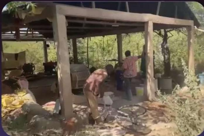
The image to the left shows local **crushing and processing** in action, where raw **ore** is converted into concentrated material suitable for **smelting**.
